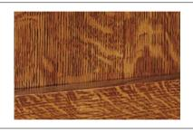
Quarter Sawn is created by using a different sawing technique to expose the different grains in the wood bringing out the flakes that remind us of family heirlooms.
